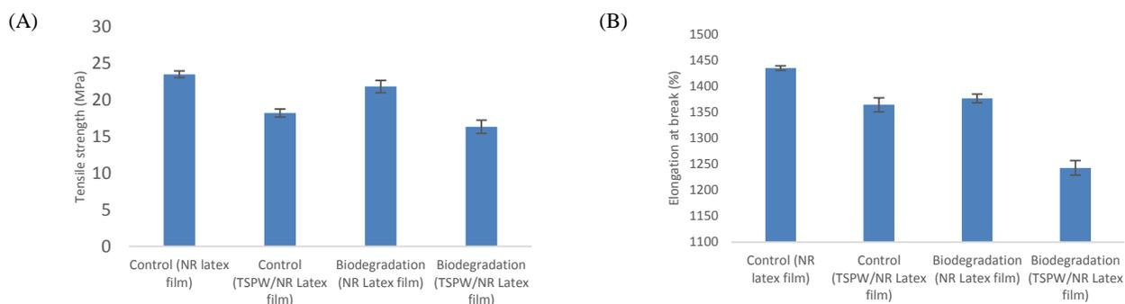
**Figure 3.** Effect of biodegradation process on films (A) tensile strength and (B) elongation at break
