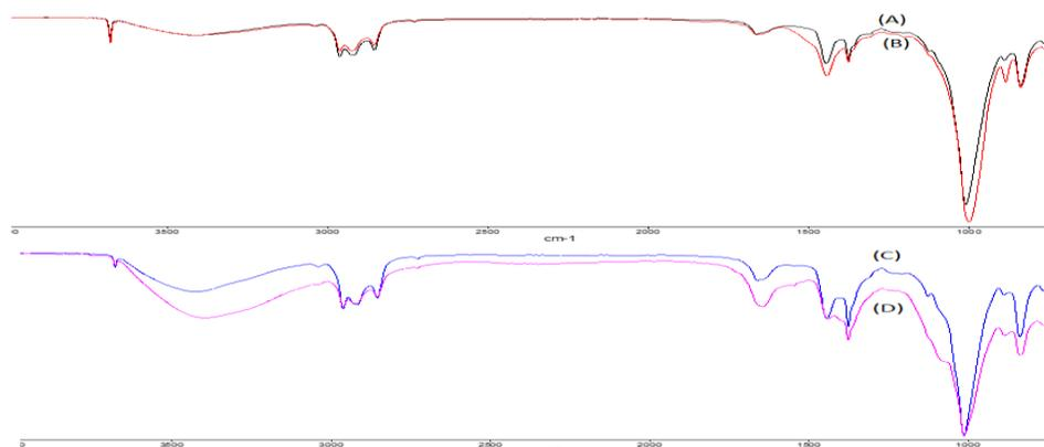
**Figure 5.** FTIR profile for different types of film with (A) Control (NR latex film), (B) Control (TSPW/NR latex film), (C) Biodegradation (NR latex film), (D) Biodegradation (TSPW/NR latex film)
