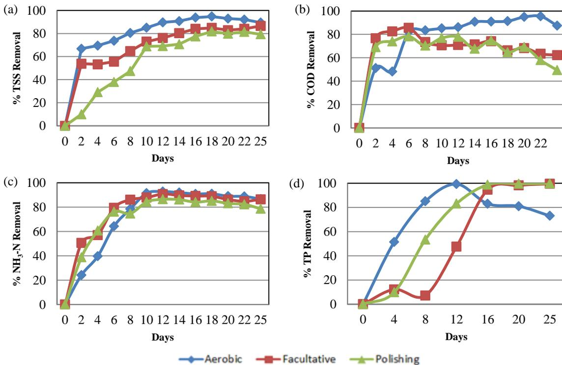
Figure 2. Removal efficiencies of the CWs during 25 days of treatment (a) TSS, (b) COD, (c)  $\text{NH}_3\text{-N}$ , (d) TP
