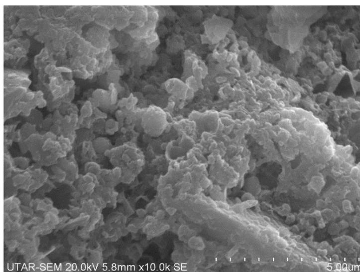
Figure 8. SEM image of EAF dust solid residue after leaching using 5M of HCl at 70°C
