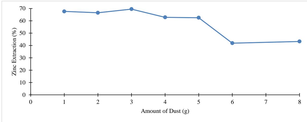
**Figure 5.** The effect of dust-to-acid ratio on zinc extraction
