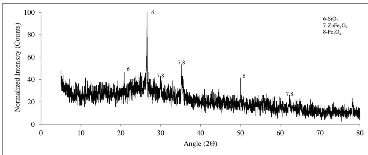
Figure 7. XRD analysis of EAF dust solid residue after leaching using 5M of HCl at 70°C
