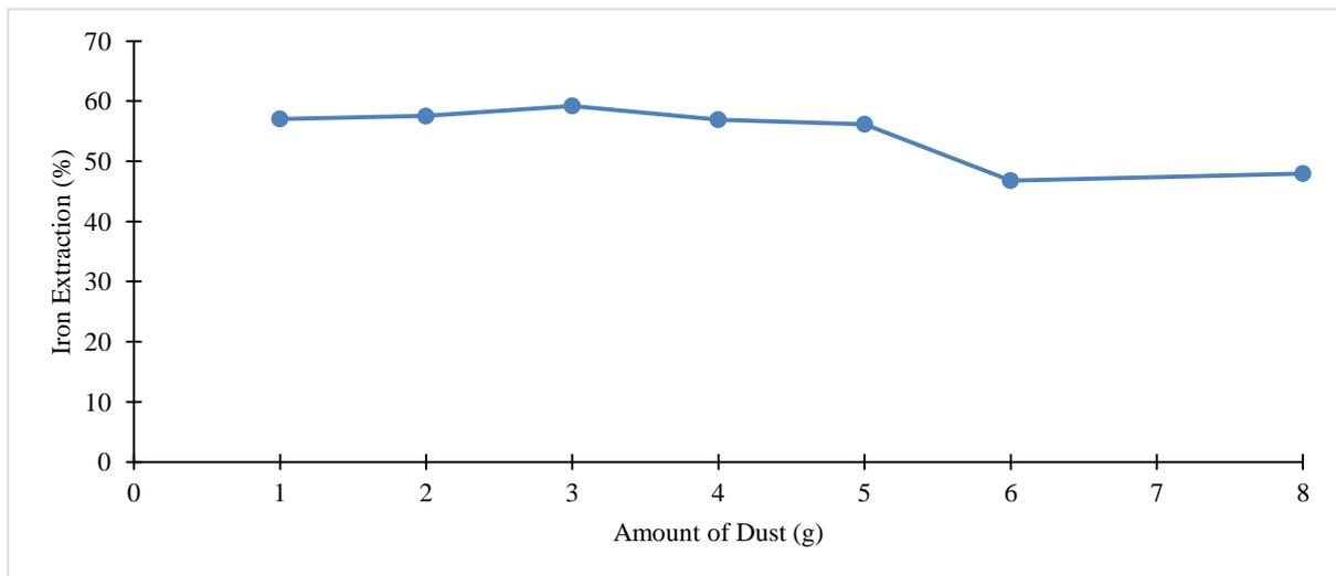
**Figure 6.** The effects of dust-to-acid ratio on iron extraction
