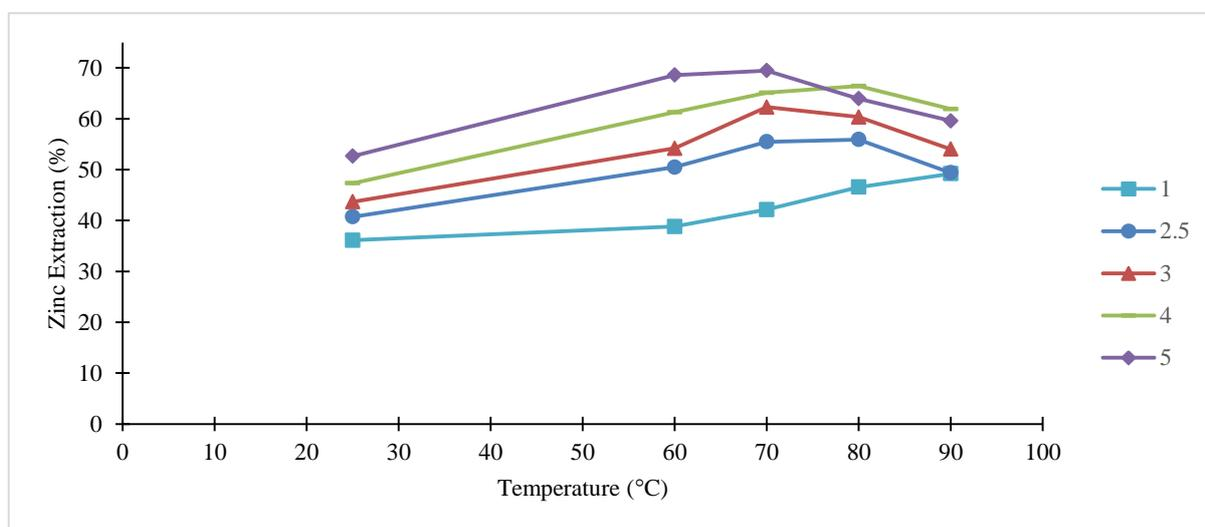
**Figure 3.** The effects of acid concentration and temperature on zinc extraction
