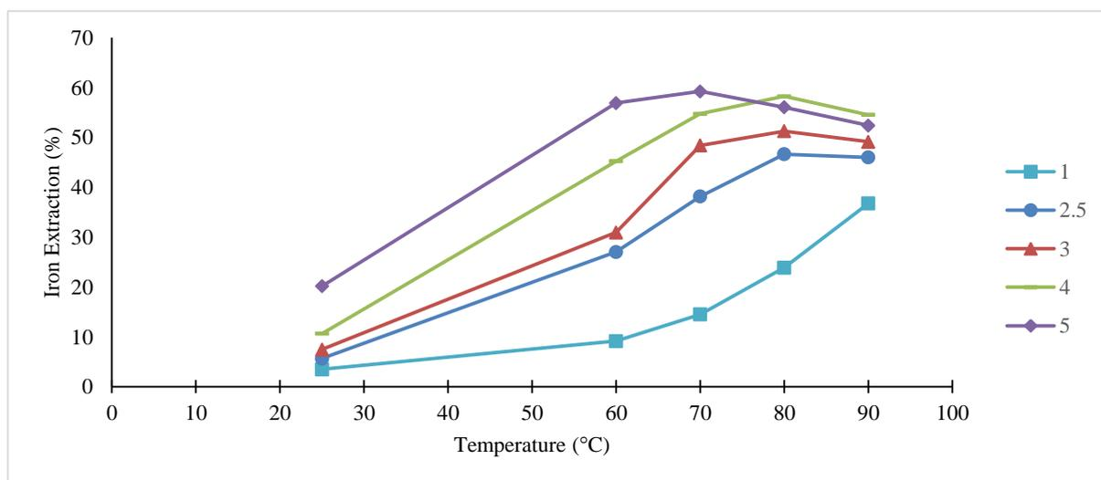
**Figure 4.** The effects of acid concentration and temperature on iron extraction
