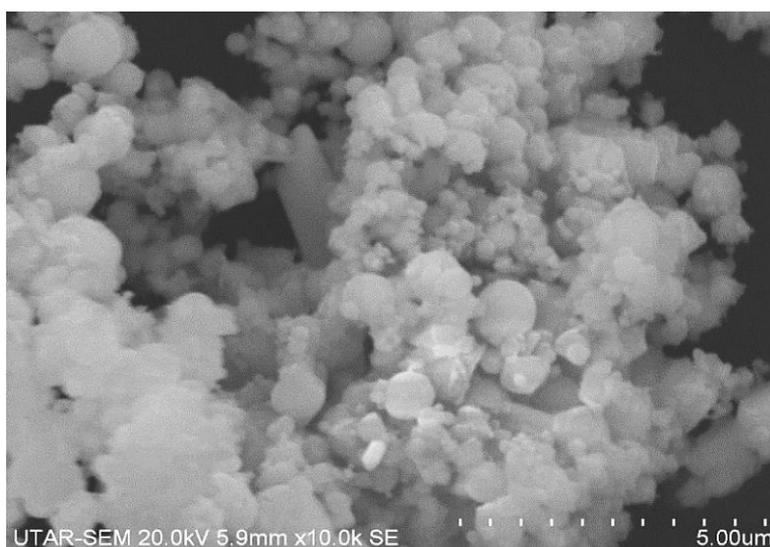
Figure 2. SEM image of EAF dust
