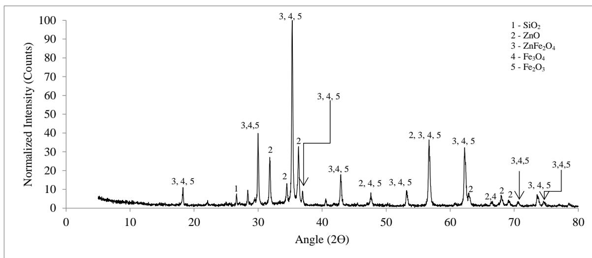
Figure 1. XRD analysis of EAF dust
