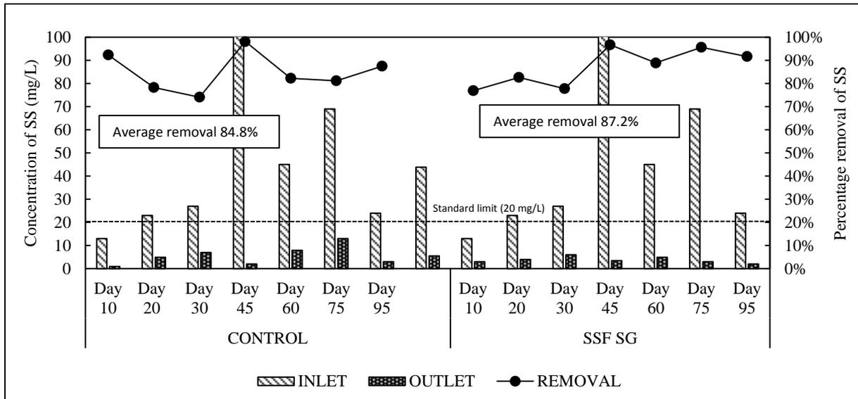
Figure 5. Variation of suspended solids between subsurface control and subsurface *S. grossus*
