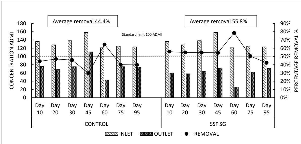
Figure 4. Variation of colour between subsurface control and subsurface *S. grossus*
