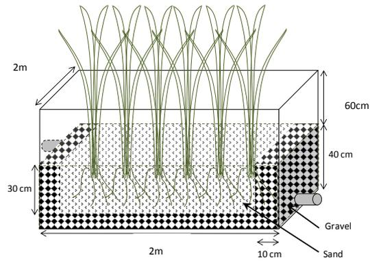
Figure 1. Size and arrangement of gravel and sand in subsurface flow with *Scirpus grossus*
