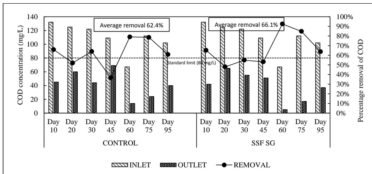
Figure 3. Variation of COD between subsurface control and subsurface *S. grossus*
