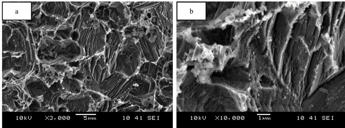
**Figure 2.** SEM images of (a) ZnO anodized on Zn foil photoanode under 0.5M phosphoric acid with x3 000 magnification, (b) ZnO anodized on Zn foil photoanode under 0.5M phosphoric acid with x10 000 magnification for 2 hours
