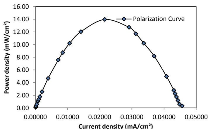
Figure 5. Power density curves of hybrid system of PFC and Fenton process
