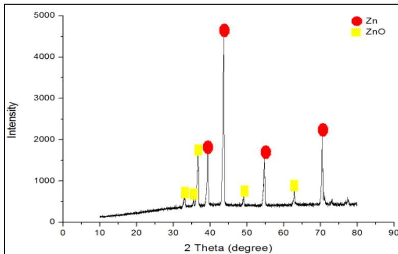
**Figure 3.** XRD pattern of anodized ZnO/Zn photoanode
