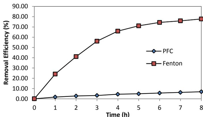
Figure 6. RB5 removal efficiency of PFC and electro-Fenton reactor
