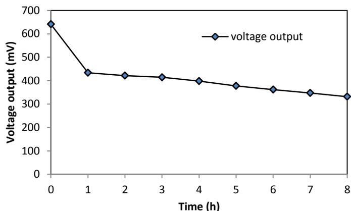
Figure 4. Voltage output of hybrid system of PFC and electro-Fenton process
