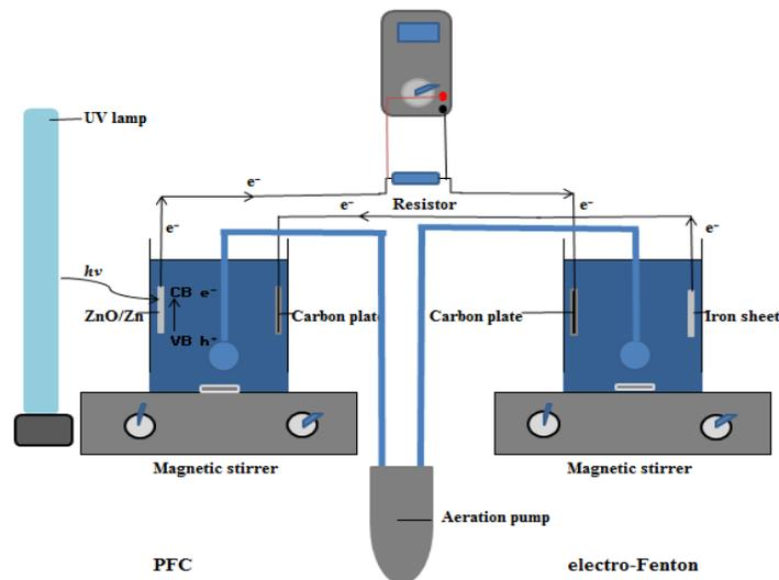
Figure 1. Schematic diagram of hybrid system of PFC and Fenton process
