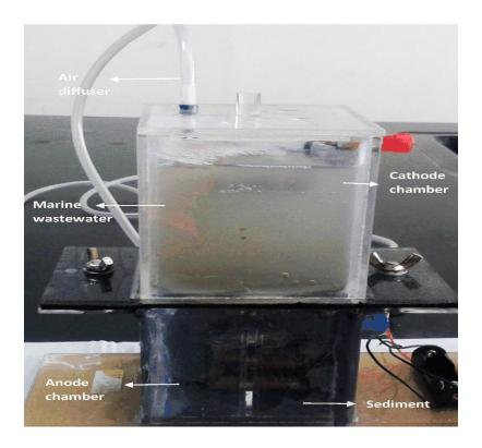
Figure 1 Prototype of SMFC
