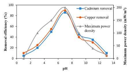
Figure 4 The effect of pH on the performance of SMFC
