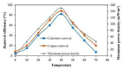
Figure 5 The effect of temperature on the performance of SMFC
