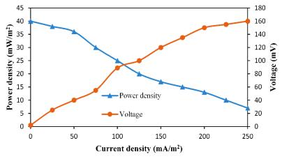
Figure 3 Polarization curve of SMFC
