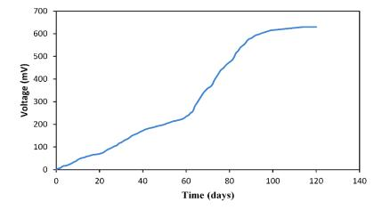
Figure 2 Voltage measurement of SMFC
