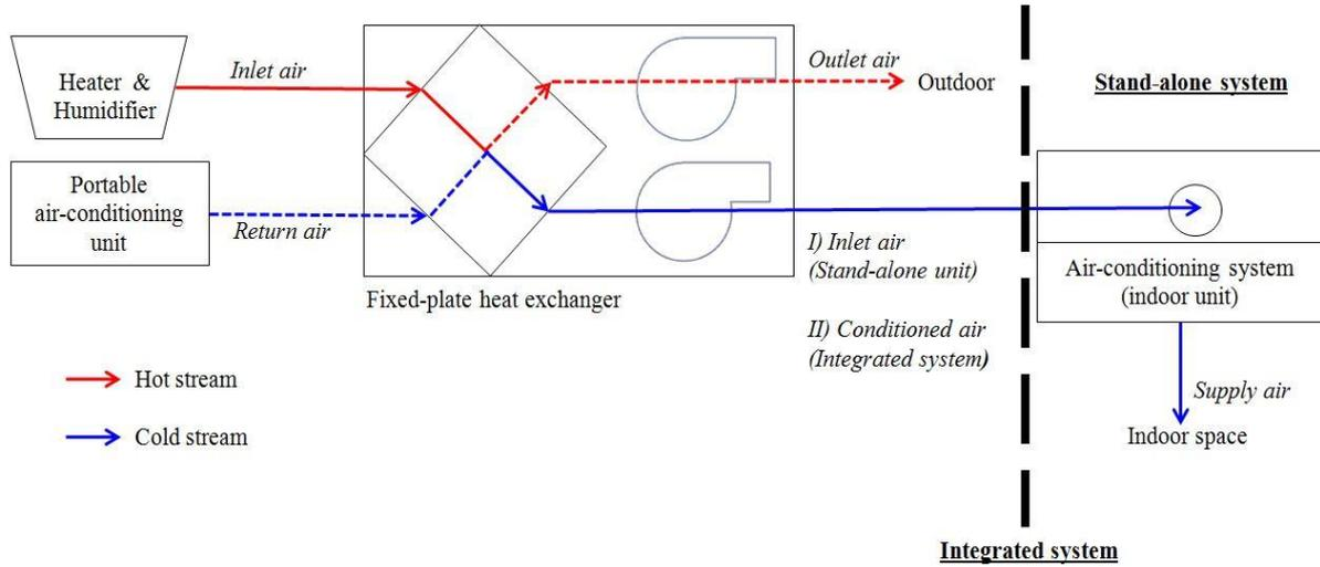
**Figure 1** Experimental set up of stand-alone and integrated system.
