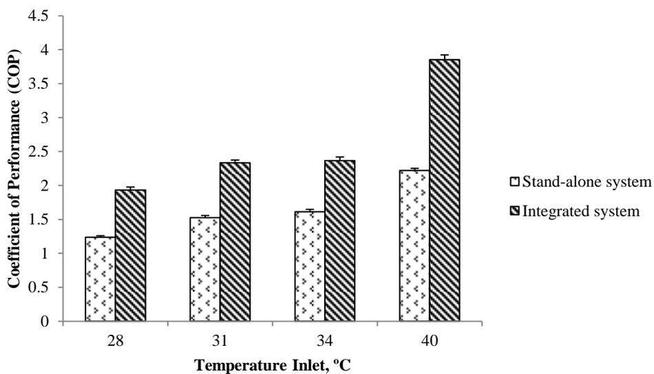
**Figure 3** Comparison of coefficient of performance (COP) between stand-alone and integrated system.
