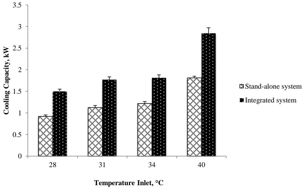
**Figure 2** Comparison of cooling capacity between stand-alone and integrated system.
