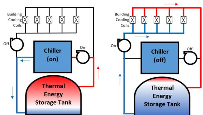
Figure 1 Off peak cooling mode (left) and peak rate cooling mode (right)
