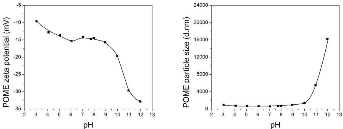
**Left: Figure. 1 (a)** shows the change in zeta potential of POME in response to pH adjustment on the suspension from 3 to 12
