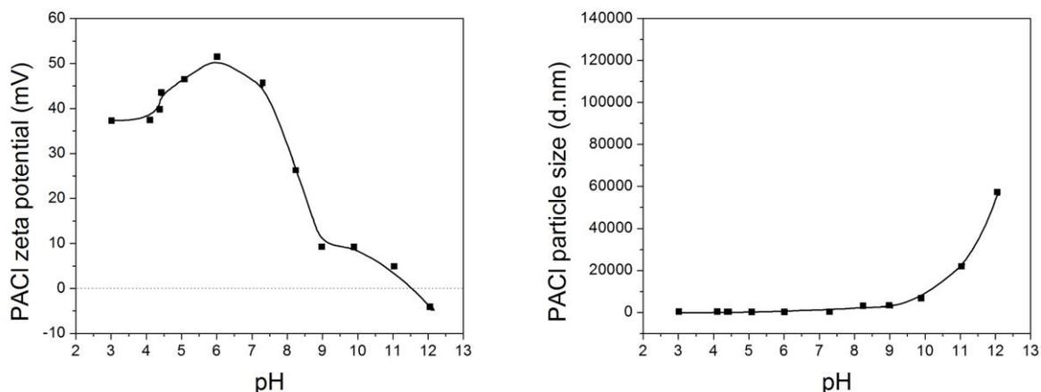
**Left: Figure. 2 (a)** shows the zeta potential profile of PACl as a function of pH within pH range from 3 to 12
