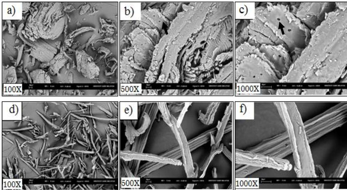
**Figure 1.** SEM micrographs of (a), (b), (c) raw *Rhizophora apiculata* and (d), (e), (f) microcrystalline cellulose after acid hydrolysis
