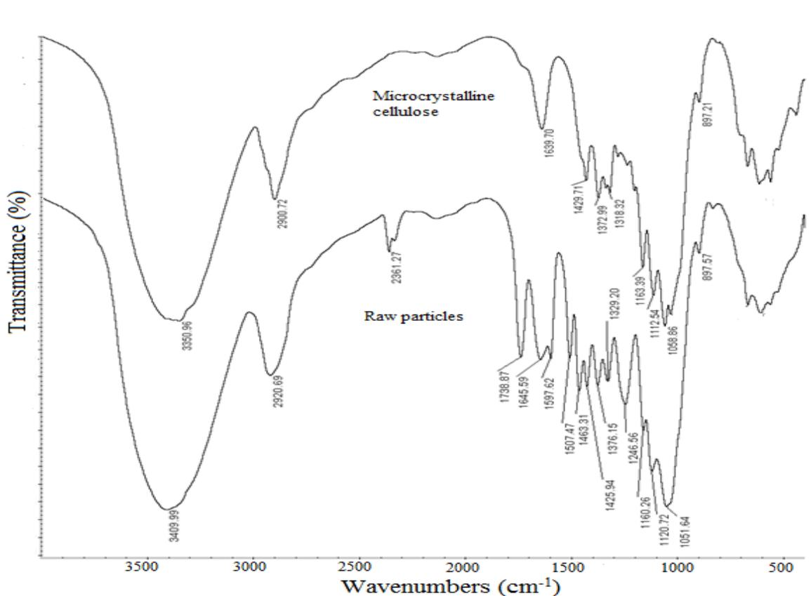
**Figure 3.** FTIR spectra of raw particles and microcrystalline cellulose of *Rhizophora apiculata*
