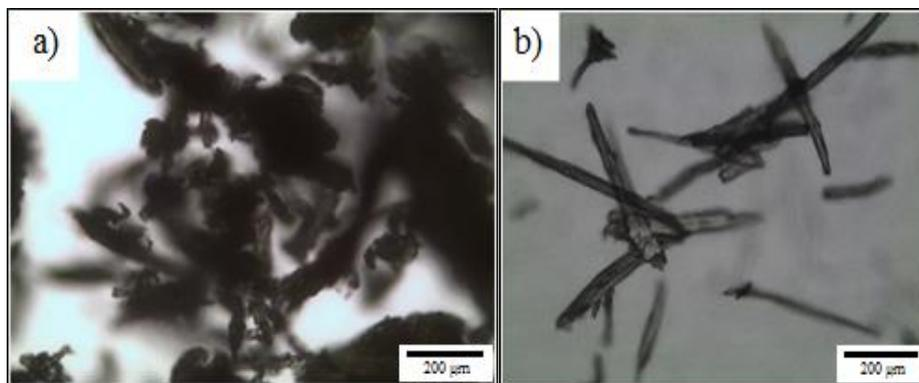
**Figure 2.** Light microscope of a) raw particles and b) microcrystalline cellulose
