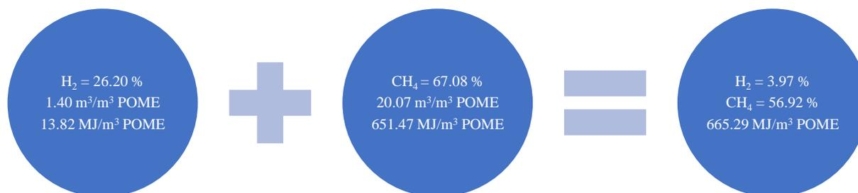
**Figure. 2** Biohythane and energy production from two-stage AD of POME.
