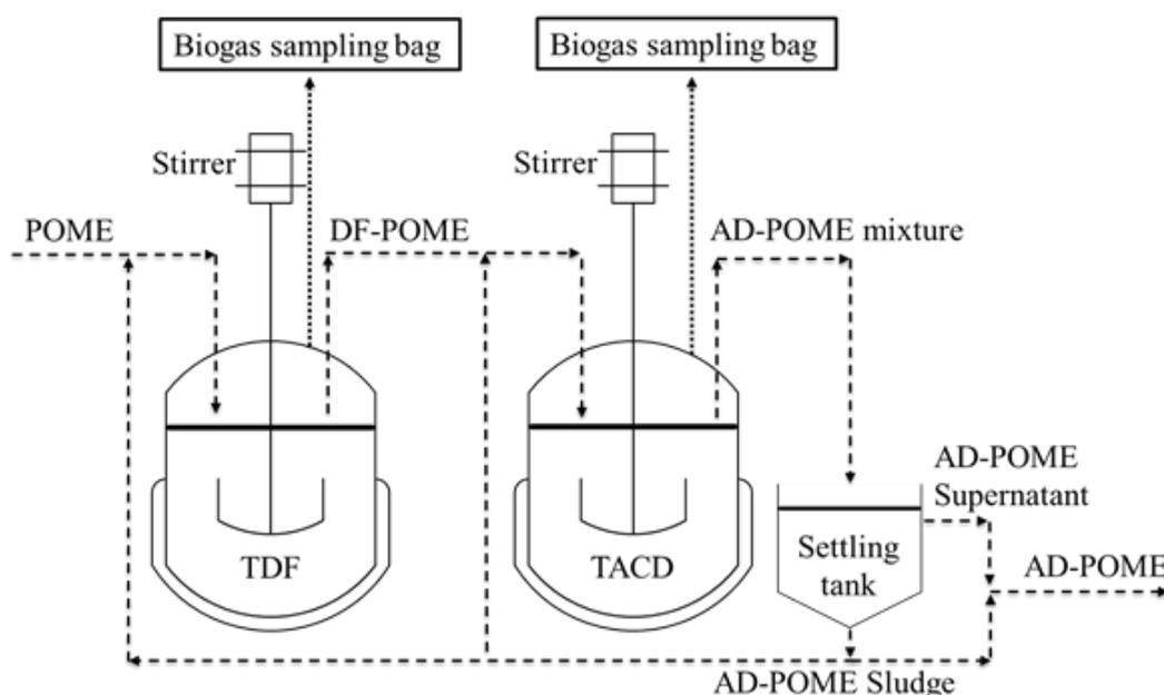
Figure 1. Schematic diagram of two-stage AD of POME.
