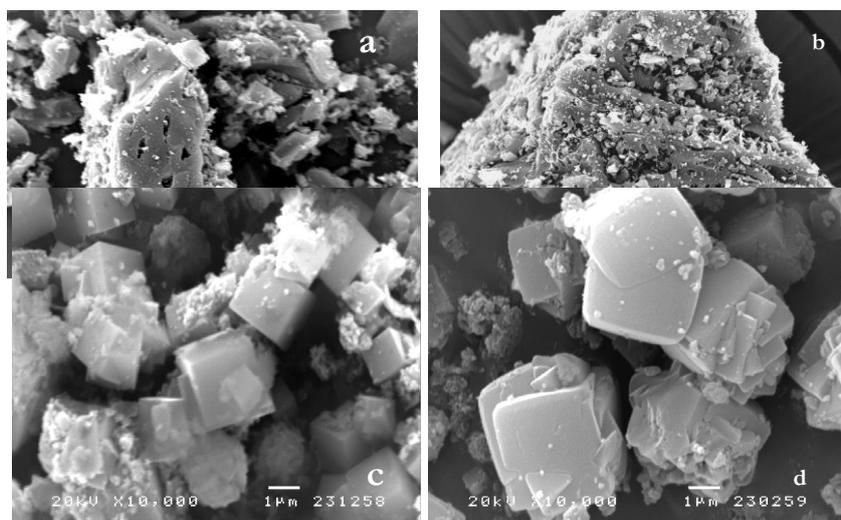
Figure 2. SEM images of (a) GAC, (b)  $\text{CMS}_{\text{GAC}}$  (PEI/CVD/GAC), (c) zeolite 5A and Li-5A zeolite.
