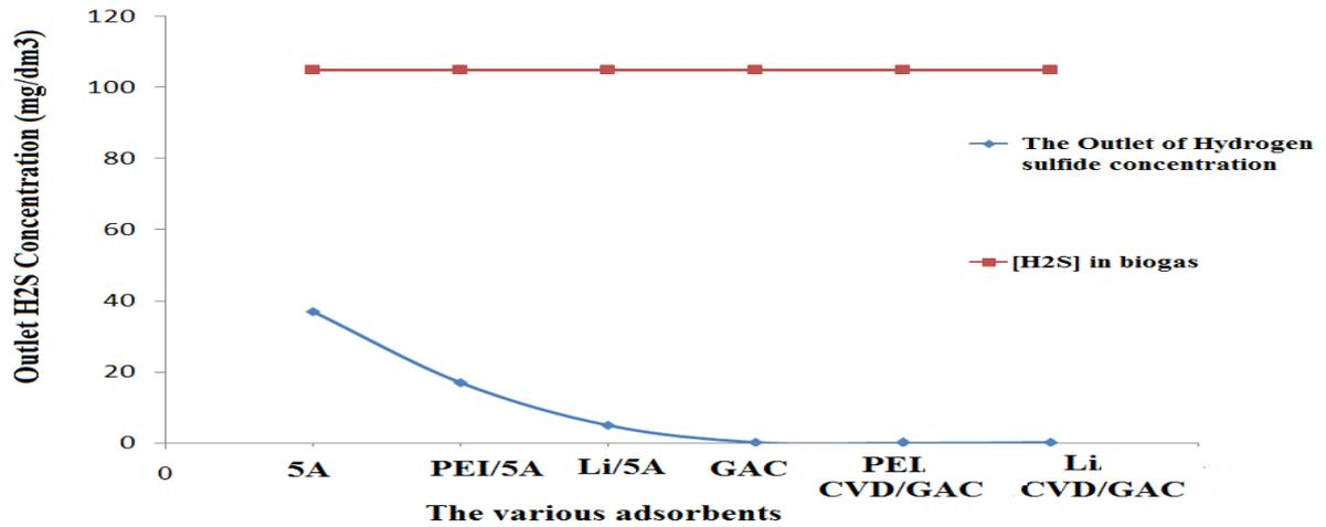
**Figure 6.** The outlet H<sub>2</sub>S concentration in the synthetic biogas by using various adsorbent (GAC, CMS<sub>GAC</sub> (PEI/CVD/GAC), CMS<sub>GAC</sub> (Li/CVD/GAC), Zeolite 5A, Li-Zeolite 5A and PEI/Zeolite5A)
