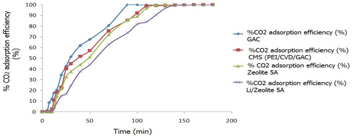
Figure 4. The breakthrough curve of the carbon dioxide adsorption efficiency by various adsorbents (GAC, Zeolite5A CMS<sub>GAC</sub>, and Li-zeolite 5A)
