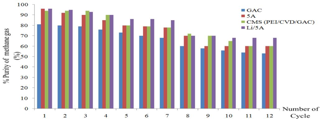
Figure 5. The purity of methane (CH<sub>4</sub>) in synthesis mixed gas by various adsorbents (GAC, Zeolite 5A, CMS<sub>GAC</sub>, and Li-Zeolite 5A )
