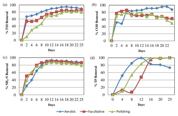
Figure 2. Removal efficiencies of the CWs during 25 days of treatment (a) TSS, (b) COD, (c) NH<sub>3</sub>-N, (d) TP
