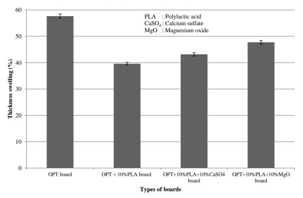
Figure 1: Thickness swelling of oil palm trunk particleboards.
