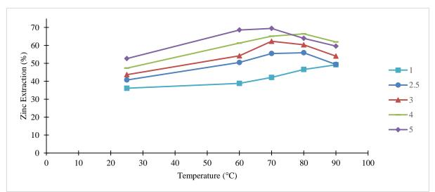
Figure 3. The effects of acid concentration and temperature on zinc extraction
