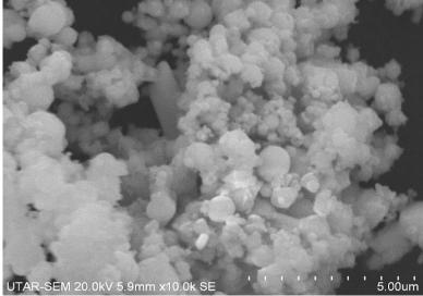
Figure 2. SEM image of EAF dust
