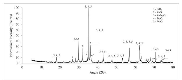
Figure 1. XRD analysis of EAF dust
