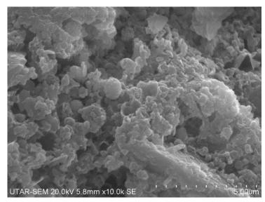
Figure 8. SEM image of EAF dust solid residue after leaching using 5M of HCl at 70°C
