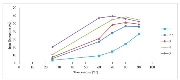
Figure 4. The effects of acid concentration and temperature on iron extraction
