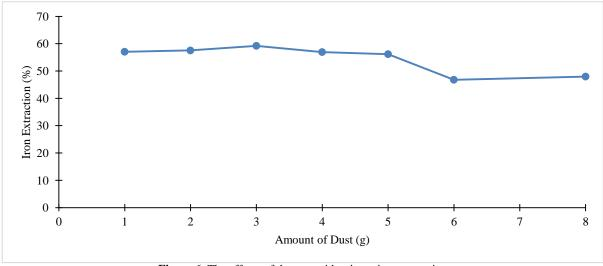
Figure 6. The effects of dust-to-acid ratio on iron extraction
