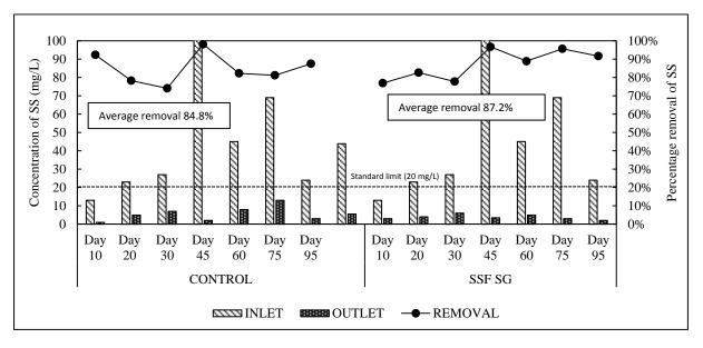
Figure 5. Variation of suspended solids between subsurface control and subsurface S. grossus
