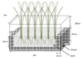
Figure 1. Size and arrangement of gravel and sand in subsurface flow with Scirpus grossuss
