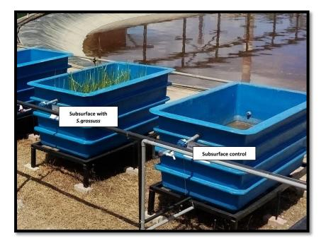
Figure 2. The pilot subsurface flow constructed wetlands developed in MNI
