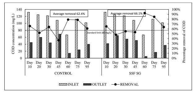
Figure 3. Variation of COD between subsurface control and subsurface S. grossuss
