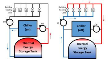
Figure 1 Off peak cooling mode (left) and peak rate cooling mode (right)
