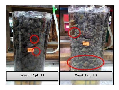
(a) (b) **Figure 1**. Adsorption mechanism on surface of steel slag in pH 11 (a) and precipitation mechanism at the bottom of the filter in pH 3, high Fe steel slag system
