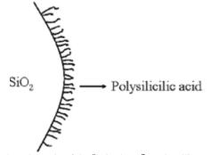
Figure 2. The schematic of the "hairy layer" on the silica particle surface [11].
