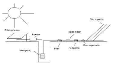
Figure. 2: Typical set-up of photovoltaic (PV) driven drip irrigation system
