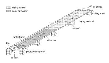
Figure 4. Solar tunnel dryer for direct solar drying with forced convection [20].
