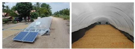
Figure 5. Inflatable solar dryer (ISD) from outside (left) and inside (right)
