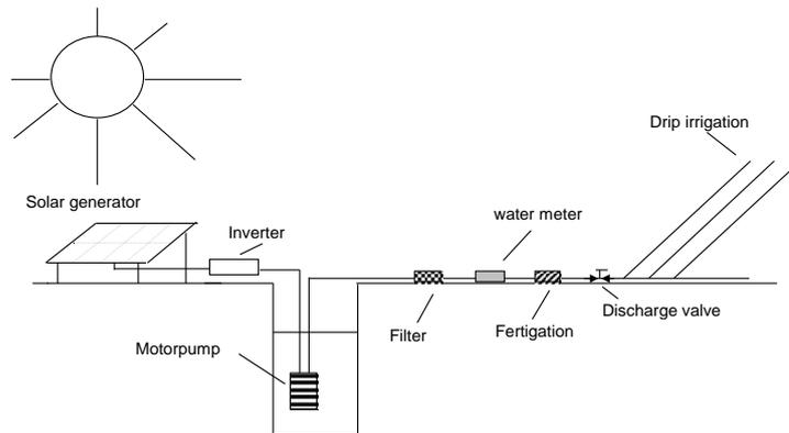
**Figure. 2:** Typical set-up of photovoltaic (PV) driven drip irrigation system
