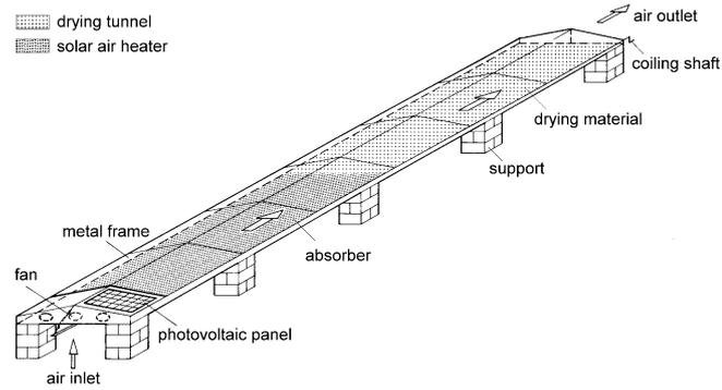
**Figure 4.** Solar tunnel dryer for direct solar drying with forced convection [20].
