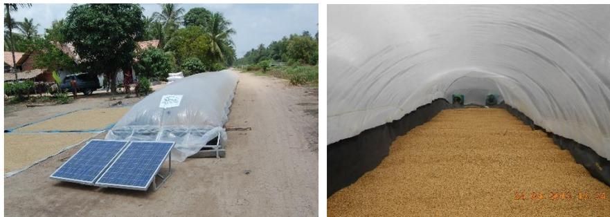
**Figure 5.** Inflatable solar dryer (ISD) from outside (left) and inside (right)
