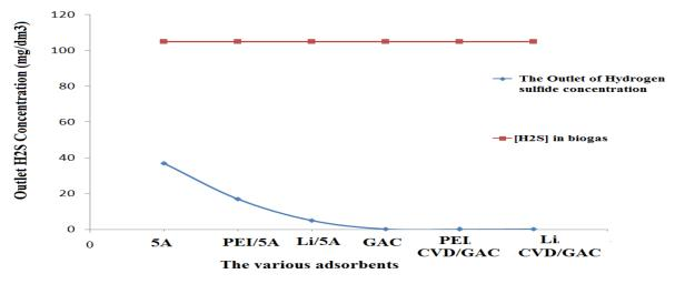
**Figure 6**. The outlet H<sub>2</sub>S concentration in the synthetic biogas by using various adsorbent (GAC, CMS<sub>GAC</sub> (PEI/CVD/GAC), CMS<sub>GAC</sub> (Li/CVD/GAC), Zeolite 5A, Li-Zeolite 5A and PEI/Zeolite5A)
