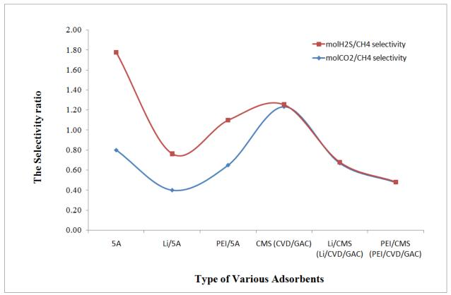
Figure 7. The Selectivity ratio by using the various adsorbents (Zeolite 5A, Li/5A, PEI/5A, GAC, Li/CMS<sub>GAC</sub>, (Li/CVD/GAC) and PEI/CMS (PEI/CVD/GAC)
