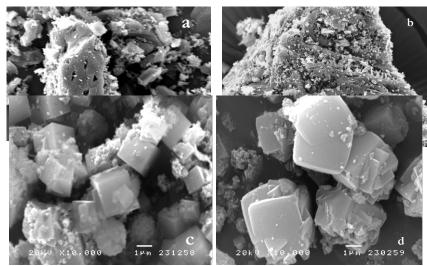
Figure 2. SEM images of (a) GAC, (b) CMS<sub>GAC</sub> (PEI/CVD/GAC), (c) zeolite 5A and Li-5A zeolite.
