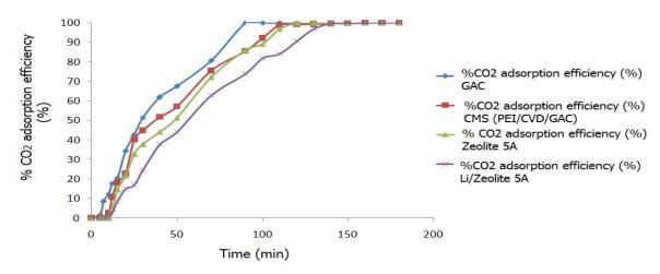
Figure 4. The breakthrough curve of the carbon dioxide adsorption efficiency by various adsorbents Zeolite5A CMS<sub>GAC</sub>, and Li-zeolite 5A) (GAC,
